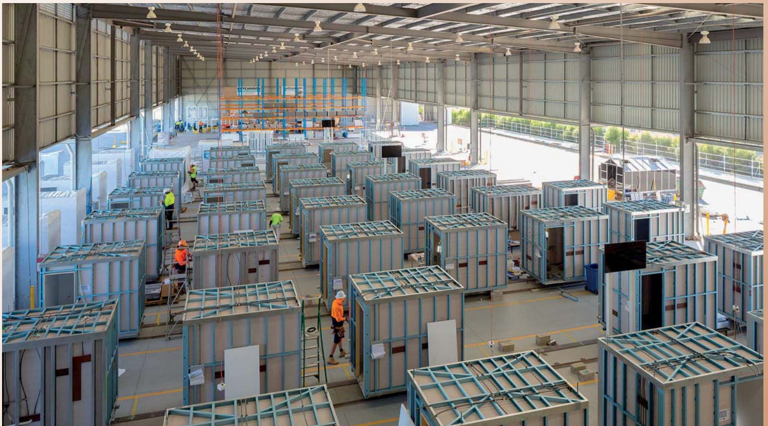
Bathroom pods manufactured in the modular factory.
